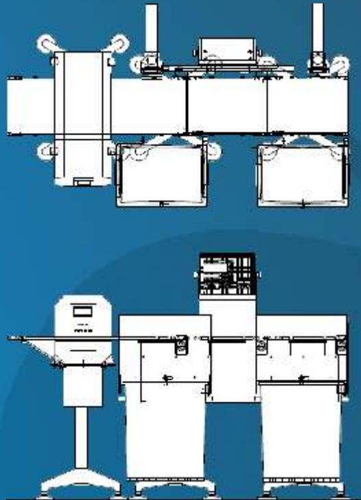
If the production demands it, the section with metal-detector is available and it can be added in a standard checkweigher: the connection with the standard checkweigher is very simple: it's enough to insert the connector and the metal-detector section is operating.
