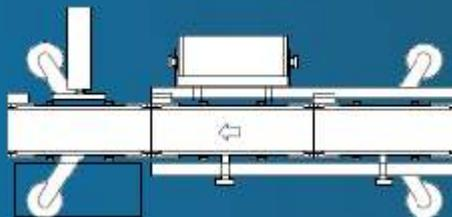
If the production demands it, the section with metal-detector is available and it can be added in a standard checkweigher: the connection with the standard checkweigher is very simple: it's enough to insert the connector and the metal-detector section is operating.
